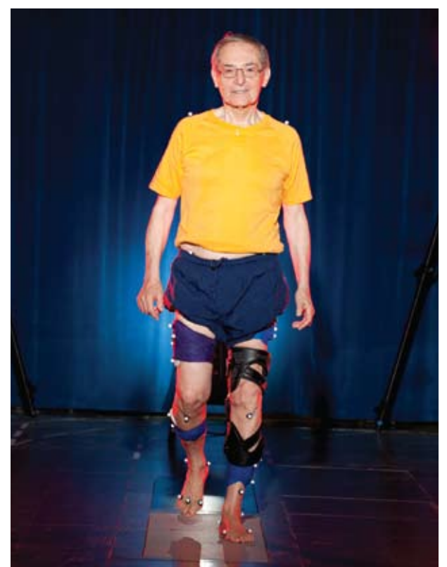
Biomechanical engineers in the Motion Analysis Lab test the effects of a knee brace on a patient with osteoarthritis.
