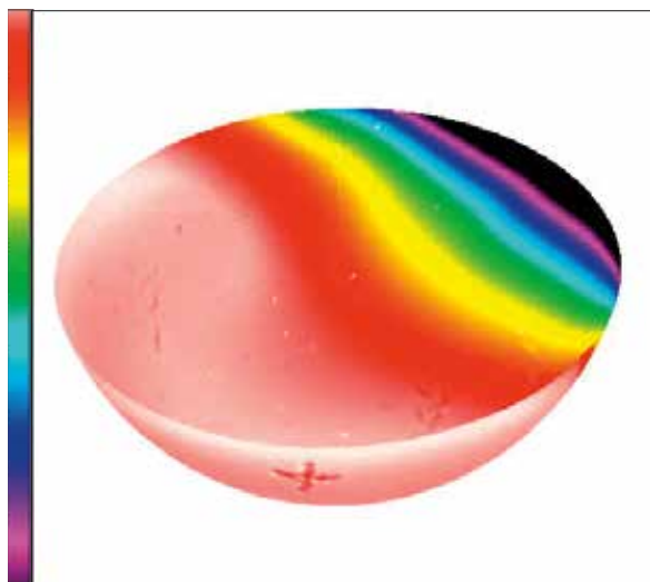
This image of a retrieved cup from a failed metal-on-metal implant maps the wear damage – colors toward the bottom of the scale (closer to black) correlate with the most wear.
