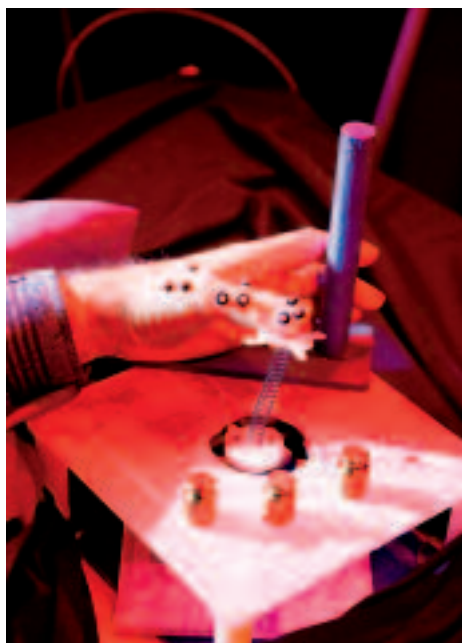
Markers placed strategically on specific areas of the hand allow the cameras to easily capture the thumb’s motion in using the strength-dexterity test device.
