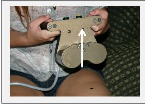
At any time during the lengthening process, you can move the Hand Piece off your leg. The motor will still run but it will not lengthen your rod.
